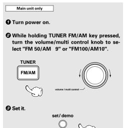
Each press switches the space frequency alternately.
