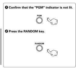
• If the **"PGM**" indicator is lit, turn it off by pressing the **PGM** key in stop mode to cancel the program mode.
